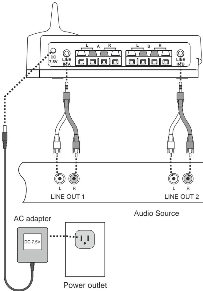
**Example 1:** Using the transmitter line-level audio inputs
