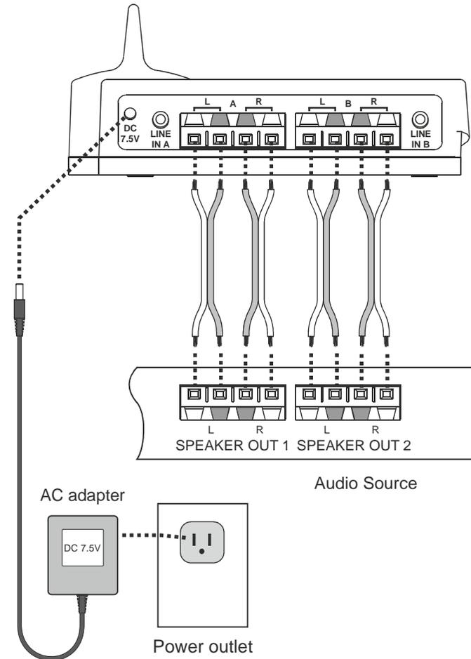
**Example 2:** Using the transmitter speaker-level audio inputs
